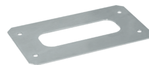
Foundation plate with anchor bolts included. Motor and floor fixing distance 269 mm x 106 mm, no. 4 Ø 12 mm.
