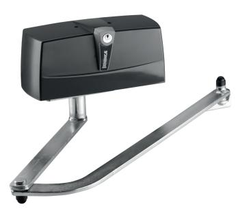
Irreversible geared motor suitable for gates installed on large columns, available in 240 Vac and 24 Vdc versions. Built-in electromechanical open and close limit switches, with sturdy articulated anti-shearing arm in galvanised steel.
