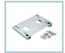
BULL.PI Raised foundation plate. Height 32 mm. Floor fixing distance 280x170 mm, no. 4 Ø 11 mm, motor fixing distance 269x106 mm n.4 M10.
